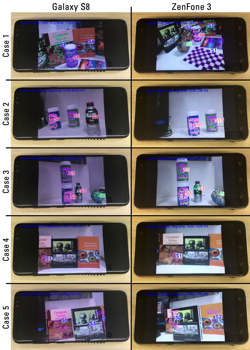
Figure 5.1: Results of GS-IST running on a Samsung Galaxy S8 and an ASUS ZenFone 3. Blue labels represent planes, green ones are for spheres and red for cylinders 4 .
