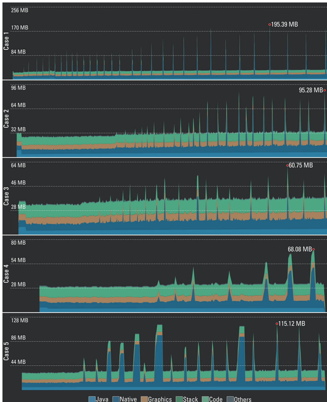
Figure 5.5: Memory usage over time of GS-IST running on ZenFone 3. Each test case has a different time scale.
