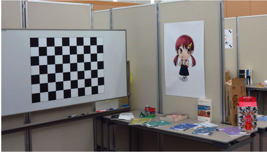
Figure 3.29: Images from the tracking area. The chessboard used to calibrate the tracking system is seen on the top left image. The other images show the tables with the trackable objects and the posters to mark the 3D points.
