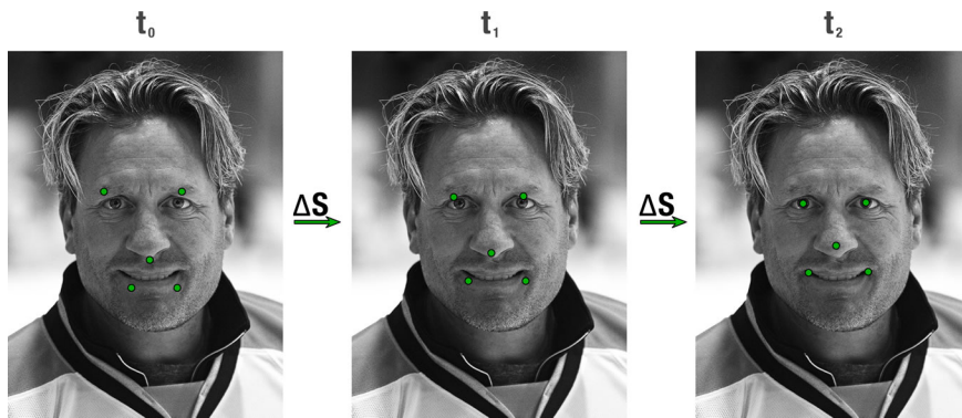
Figure 3.19: Cascade shape regressor, in which the landmark position is incremented every stage.
