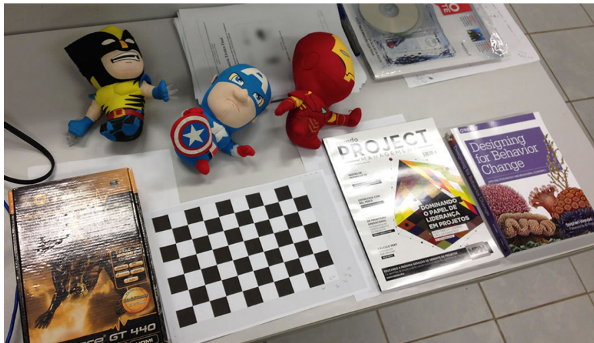
Figure 3.30: Evaluation environment with the calibration chessboard in the middle and objects with different types of texture around it.
