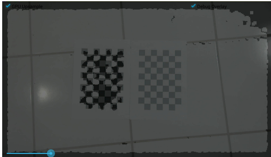
Figure 3.6: Screenshot of the depth estimation of two chessboards printed on a paper. On the right, the one printed with a mix of cyan, magenta and yellow inks. On the left, the same pattern printed with a black ink. Note that the sensor is not able to estimate depth on the black squares of the left paper.
