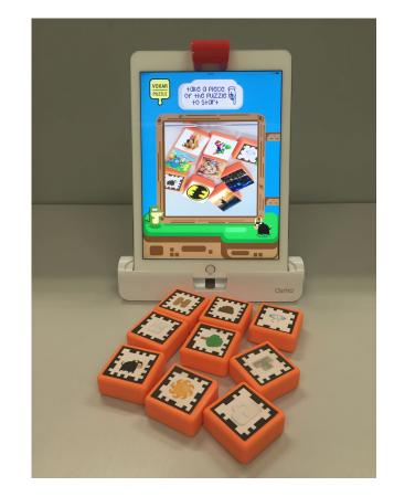
Figure 1: AR jigsaw running on Voxar Puzzle. Note that the iPad is on the Osmo's tablet support and the mirror is the red object covering the frontal camera.
