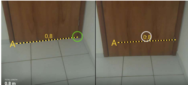
Figure 8: Door width estimation using Tango tablet. Left side shows the initial measurement and the right side shows the ruler position after moving the device. Door actual width is 0.7 meters.
