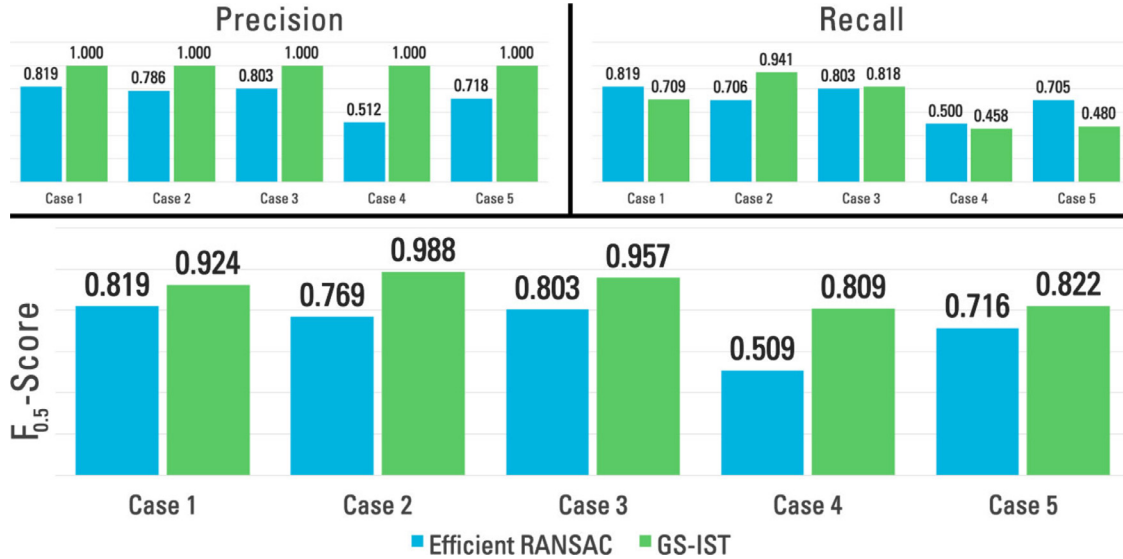
Fig. 4. Comparison of precision, recall and F_{0.5} -Score between Efficient RANSAC [20] and GS-IST.
