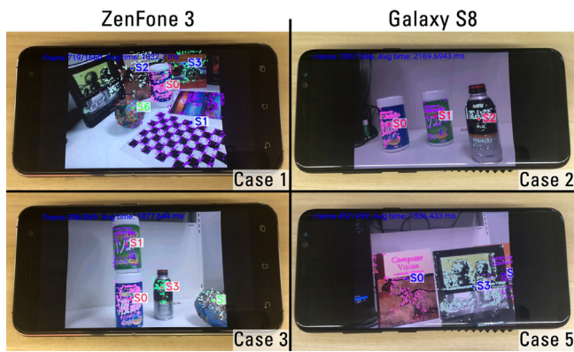
Fig. 10. Results of GS-IST running on a Samsung Galaxy S8 and an ASUS ZenFone 3. Blue labels represent planes, green ones are for spheres and red for cylinders. (For interpretation of the references to color in this figure legend, the reader is referred to the web version of this article.)
